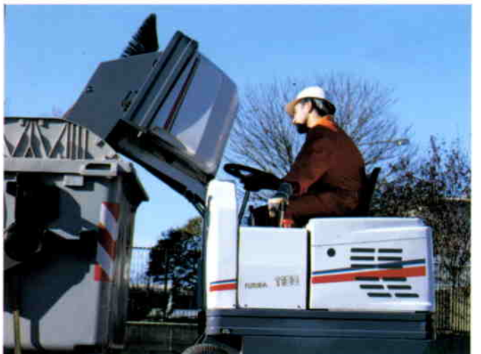
Emptying the waste hopper
