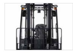
The neatly arranged hydraulic hoses and chains provide clear front visibility through the wide view mast.
