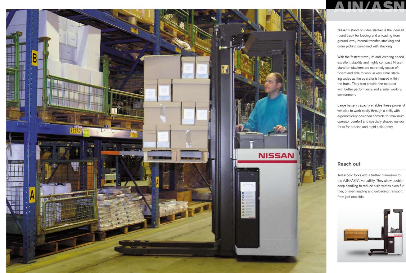
Nissan's stand-on rider-stacker is the ideal all round truck for loading and unloading from ground level, internal transfer, stacking and order picking combined with stacking.
